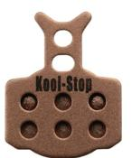
The sintered metal disc brake pads are designed to give you performance braking in extreme conditions, e.g. XC, downhill, trials and dual slalom riding. Our pads have a quick break-in period so you get maximum performance during those demanding rides when stopping power, durability and long pad life are required. Sintered metal should not be used on ceramic rotors or in closed hydraulic systems.
