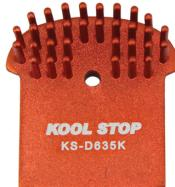
The Aero Kool disc pads are made with a forged aluminium cooling pinned backing plate and a high performance organic compound. The new pads greatly reduce heat build-up in the braking system and provide superior, lasting brake power.
