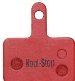
The standard disc pads are made from organic materials that are blended and bound together using a resin. The compound does include small amounts of copper which improves the braking formula.
